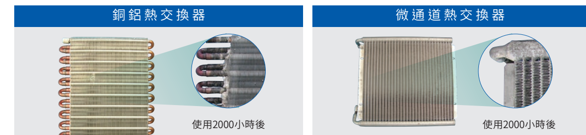
銅片腐蝕損壞 • Accelerated Salt Spray Test (SST) conditions: JIS Z 2371.
